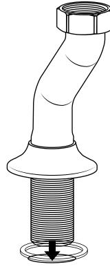
\*Remember to install the 'O' ring o washer between the mixer body & sanitary ware\*
