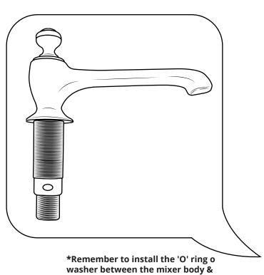
\*Remember to install the 'O' ring o washer between the mixer body & sanitary ware\*
