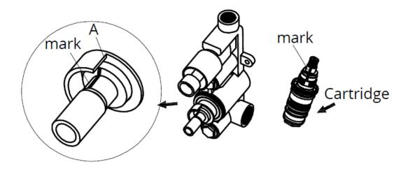
4. Fit the stop lug and handle body with part A and B aligned. Then screw and tighten the lever handle. once complete the unit is ready for use.
