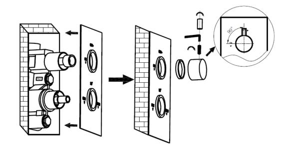
2. Secure the concealing plate to the valve body followed by the rubber washer, handle body, grub screw and hand lever.
