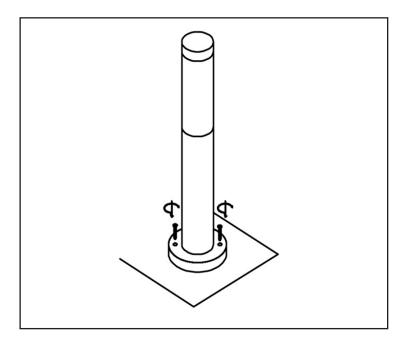
Offer the post to the ground and fix in place with the supplied screws.
