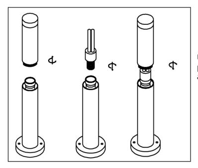
Unscrew the upper section of the post, screw in the lightbulb and reattach the upper section.
