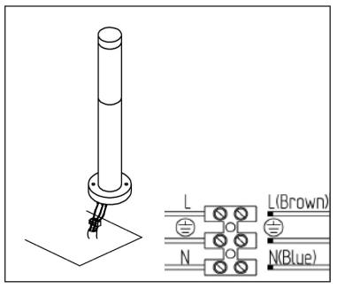
Feed the mains cable up through the ground at your chosen fixing location ,feed it through the centre of the ground spike and connect as shown.
