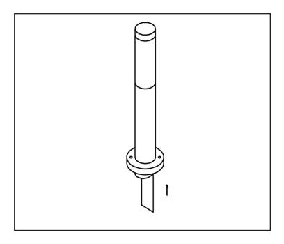
Push the ground spike back into the body of the post.
