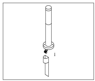
Remove the ground spike from the main body of the post lamp
