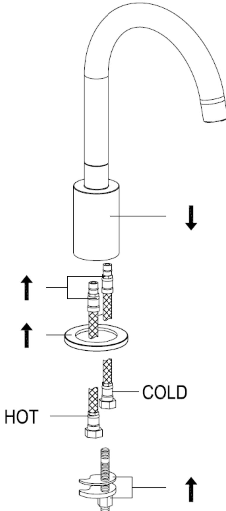
\*Remember to install the 'O' ring or washer between the mixer body & sanitary ware\*
