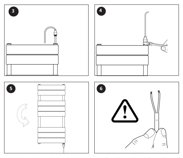
The towel rail can now be turned over so the heating element is facing downwards ready for installing on the wall.
