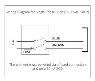
The heating element can be installed in bathrooms in zone 1, 2 and outside the zones as defined by applicable law, subject to any additional regulations concerning electrical installations in wet areas.
