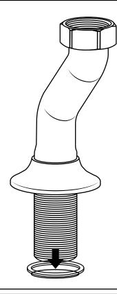
\*Remember to install the 'O' ring or washer between the mixer body & worktop\*
