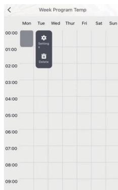
B. You can choose the weekly program or timer. The set temperature must be higher than the currently temperate.
