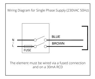
If using a thermostat with the towel rail please refer to thermostat installation guide for wiring instructions.
