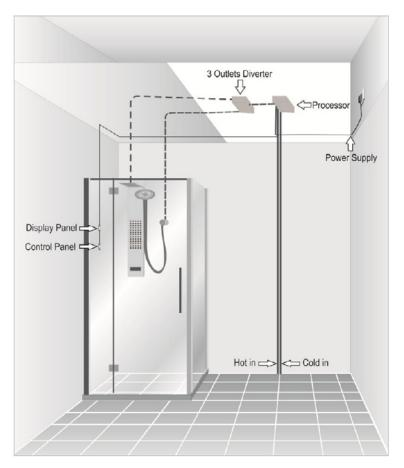
System Connection Schematic
