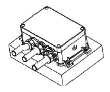
**Step 4**: The processor is fitted with copper tails. We recommend using push fit connectors for installation.
