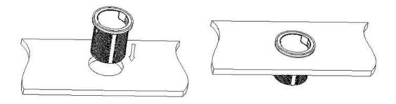
Step 3 : Screw the clamp nut onto the installation bracket to secure it to the wall.
