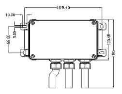
**Step 1**: Mark the fixing holes for the processor and diverter in the required position (as per the drawing on page.5)
