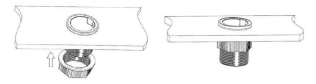
Step 4: Insert the control body and turn clockwise to lock the control panel on the wall.
