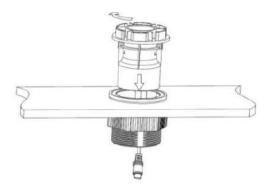
Step 5: Push the control knob onto the control body to complete.
