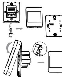
1. To remove the front cover, gently twist the screwdriver clockwise as shown.
