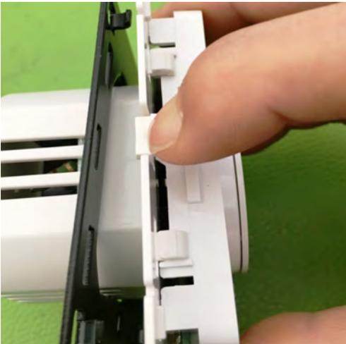
3. Fix the metal back-plate to a 38mm deep wall box, wire up the unit as shown and reassemble.
