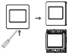
2. Take the backing plate apart according to the following diagram.
