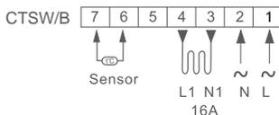
Wiring should be carried out by a qualified Electrician in accordance with I.E.E. Regulations. We do not recommend the timerstat be installed inside a bathroom or location where it can be affected by steam.
