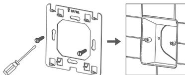
4. Connect wires (see diagram), and then mount thermostat on the backing plate and remounted the cover and frame
