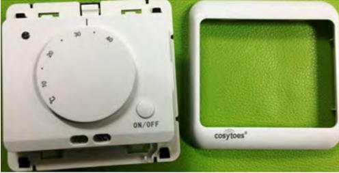
2. Use flat screwdriver to press fixing clips and detach metal back plate.
