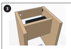
Mark out and drill the hole for your flush button, making sure that it will not foul against the cistern once fitted.
