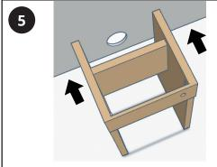
Once you have decided on the location of the unit, offer it to the wall, making sure the soil pipe is as central as possible and fasten the frame to the wall via the fixing brackets.
