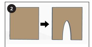
Using your purchased toilet as a template, cut a hole in the lower panel to allow for the flush pipe and waste pipe, but is still small enough for  $% \left\{ 1\right\} =\left\{ 1\right\} =$ the toilet to cover.
