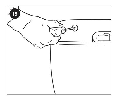
Drill holes for the marked floor mounting screws, again inserting suitable wall plugs for the required surface.
