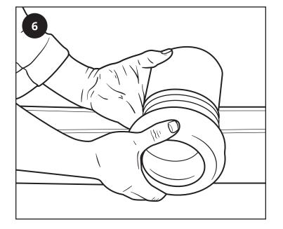
Insert your pan connector into the waste pipe making sure it fits snugly and is sealed all the way around .
