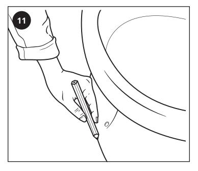
Pull the toilet away from the wall. Drill the previously marked cistern fixing holes and use suitable wall plugs for the surface in question
