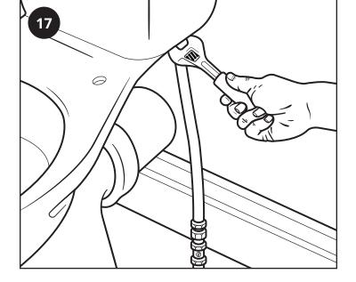
Open the isolation valve on the water pipe, check for leaks at any of the pipe joints, flush the WC and check the pan connector for leaks.
