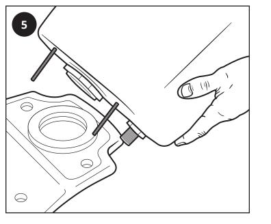
Place the close coupled washer carefully in position making sure it is correctly lined up.
