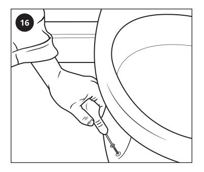
Fix the pan to the ground with fixing screws again using any provided washers.
