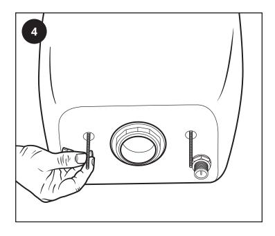
Feed the connecting bolts through the inside of the cistern making sure that the provided washer are added to keep the cistern water tight.
