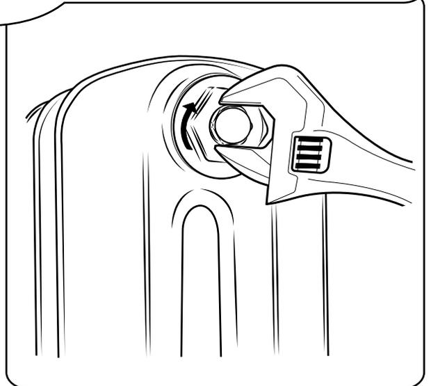
**i** Do not over tighten or it may cause leaks
