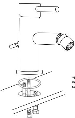
\*Remember to install the 'O' ring or washer between the mixer body & sanitary ware\*
