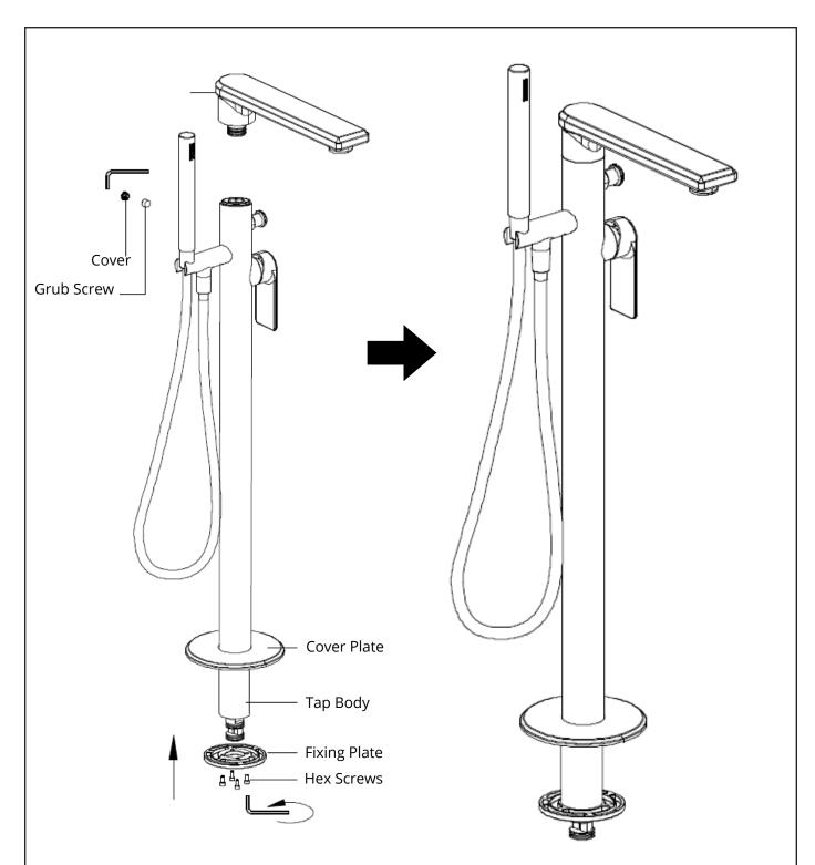
Place the cover plate onto the tap body and mount the fixing plate onto the end of the tap body and secure in place with the Hex head screws.
