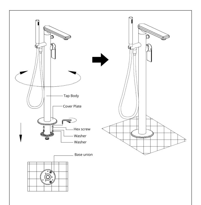
Mount the tap body onto the base union and secure in place with the hex screws and washers ,
