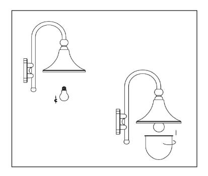
Insert lightbulb and secure bulb holder in place, the unit is now ready for use.
