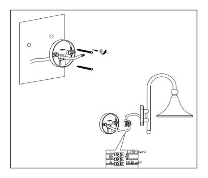
Feed the mains cable through the wall fixing plate, and connect to the terminal block on the light fitting as shown.
