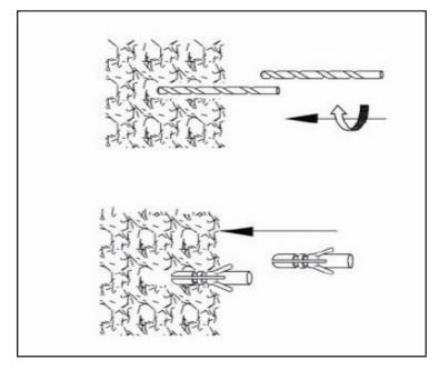
Drill out your fixing holes and insert wall plugs.
