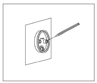
Choose a suitable fixing location ensuring that they will not be exposed to constant running water.
