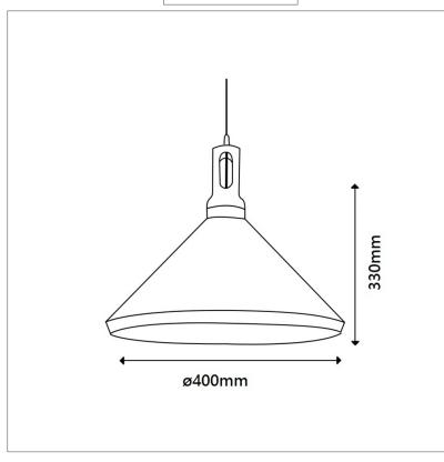
**E27** Base Dimensions ø400 x 330 mm Waterproof IP20 Input Power 220-250V Certification CE, RoHS, LVD Input Frequency 50-60HZ Weight 1kg
