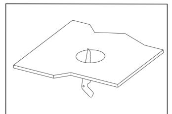
Using the Installation Spacing guide on Page 2, cut out the correct size hole for the downlight.
