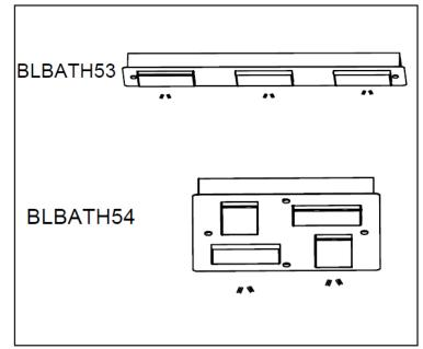
The BLBATH53 has two fixing screws to attach to the ceiling plate, the BLBATH54 has four.
