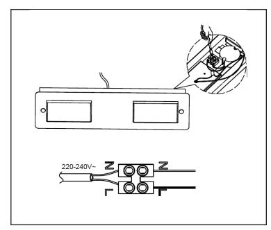
Connect the power cable to the wiring block as shown.
