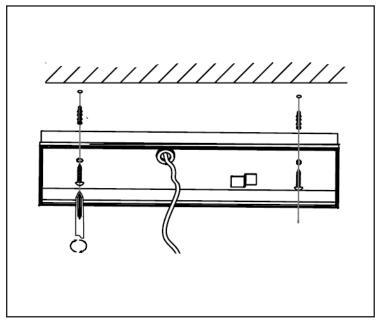
Mount the ceiling box using the provided fixings.
