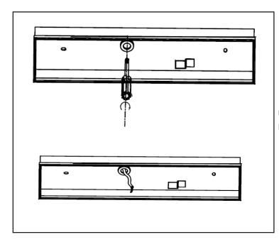
use a screwdriver to puncture a hole in the ceiling-mounting box, then feed through the power cable.
