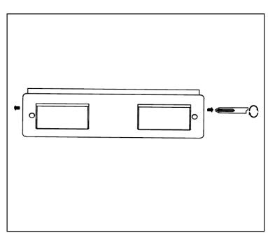
Offer the LED fitting up to the ceiling plate and fix in place with the provided screws.
