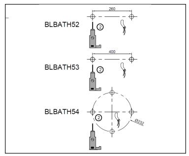
Mark out the drill centers and drill the fixing holes into the ceiling.
