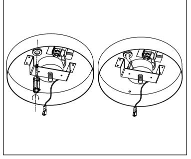
Use a screw driver to puncture a hole in the ceiling box as shown, then feed through the power cable.
