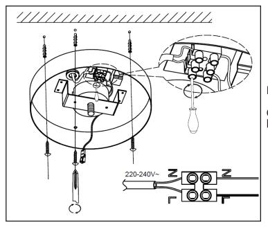
Fasten the ceiling box in place on the ceiling.
