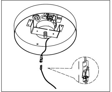
Connect the Driver cable to the cable on the LED fitting.
