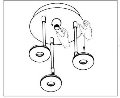
Unscrew the center retaining nut and seperate the light fitting from the ceiling mounting box.
