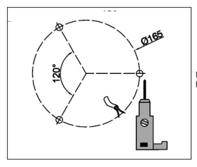
Mark out the drill centers and drill the fixing holes into the ceiling.
